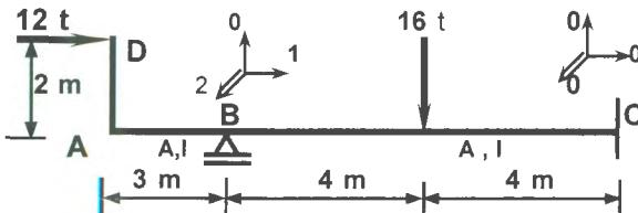
$$\begin{aligned} E &= 2000000 & t/m^2 \\ I &= 0,008 & m^4 \\ A &= 0,05 & m^2 \end{aligned}$$
